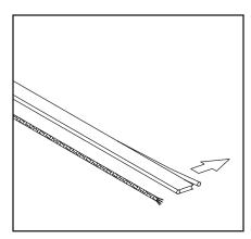
7. Starting at the end of the heating cable, using needle nose pliers or a knife pull each bus wire away from the core material. \*Separate CWM-C leads and strip 1/4" from each leadwire.
