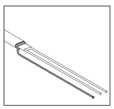
8. Remove the exposed core material and cut 1/4" of the end of each bus wire. \*Skip this step if using CWM-C constant wattage cable.
