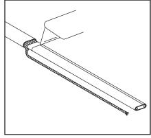
5. Score the inner insulation 6 inches from the end. Lightly cut the inner jacket up the center to end of heating cable and remove the inner jacket from the cable.
