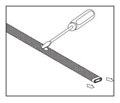
For each cable, push braiding back from the end of the cable.
