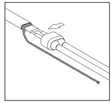
9. Liberally apply RTV over the exposed matrix and leads. Push the rubber boot over the heating cable. Trim lead ends as needed. \*Boot is not needed when using CWMC constant wattage cable.
