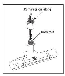
10. Slide compression fitting over cable. Grommet should be placed inside pipe standoff. Termination boot should be spaced 1/2" from sealing grommet. Tighten compression fitting until it bottoms out against pipe standoff.
