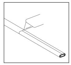
2. Score the outer insulation 7 inches from the end of the cable. Lightly cut the outer jacket up the center to the end of heating cable and remove the outer jacket from the cable. WARNING: DO NOT CUT METAL BRAID.
