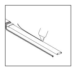
6. Shave the core material from the outside of each bus wire. \*Skip this step if using CWM-C constant wattage cable.
