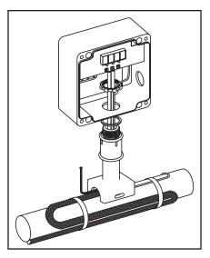
10. Assemble junction box to compression fitting as shown. Tighten locknut until the junction box bottoms out against the lip of the compression fitting.
