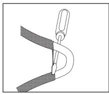
2. While bending the heating cable, work the cable through the braid opening. Pull the braid tight
