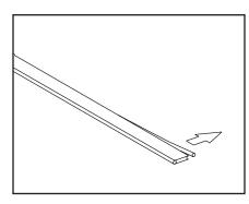
6. Starting at the end of the heating cable, using needle nose pliers or a knife pull each bus wire away from the core material. \*Separate CWM-C leads and strip 1/4" from each leadwire.
