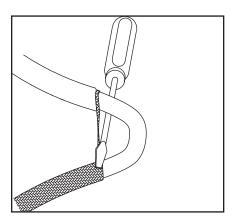
**4.** While bending the heating cable, work the cable through the braid opening. Pull the braid tight.
