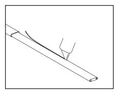
5. Shave the core material from the outside of each bus wire. \*Skip this step if using CWM-C constant wattage cable.
