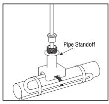
1. Insert heating cable and capillary tube through pipe standoff and grommet as shown. 8 inches of cable should extend past the grommet. Attach the pipe standoff to the pipe with a pipe strap (Chromalox type PS not included) as shown. Attach extra cable to pipe as appropriate. Small slice will need to be cut in grommet to allow the RTD wire to exit the pipe standoff out the bottom. For pipes smaller than 1-1/2" diameter optional small pipe adapter (Chromalox model SPA not included) is required.
