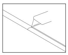
**4.** Score the inner insulation 7 inches from the end. Lightly cut the inner jacket up the center to end of heating cable and remove the inner jacket from the cable.
