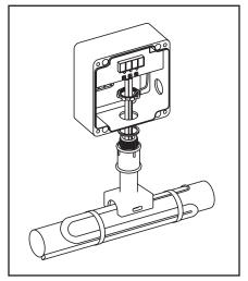
11. Assemble junction box to compression fitting as shown. Tighten locknut until the junction box bottoms out against the lip of the compression fitting.
