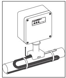
11. Attach 3/4" conduit hub. Please see the electric diagrams below for proper wiring for your application. Attach junction box cover to seal enclosure. Note: The conduit hub shall be listed for Class 1, Div. 2; Class II Div. 1 & 2, Class III, Div. 1 & 2, and 4X rated by a nationally recognized testing laboratory.
