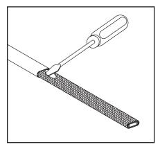
Move braid back toward the overjacket, creating a bulge. At the bulge, separate the braid to make an opening.
