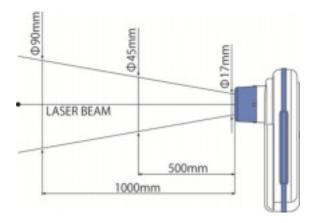
The above measuring diameter is defined as an area which allows capture of more than 90% of energy.
